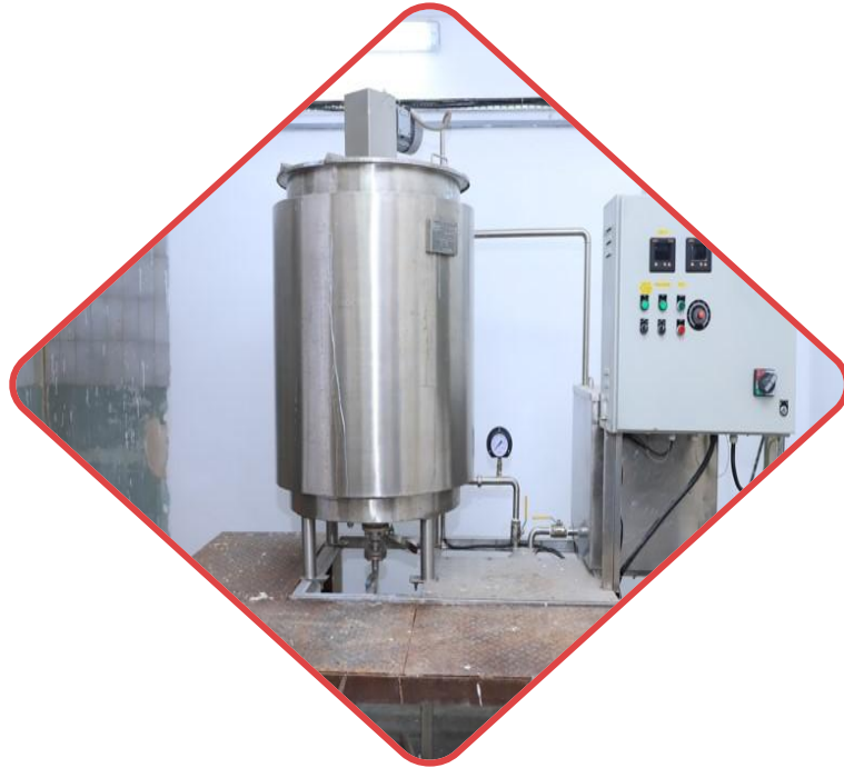
Pilot reactor of capacity 500 kg equipped with Mechanical stirring & heating facility
